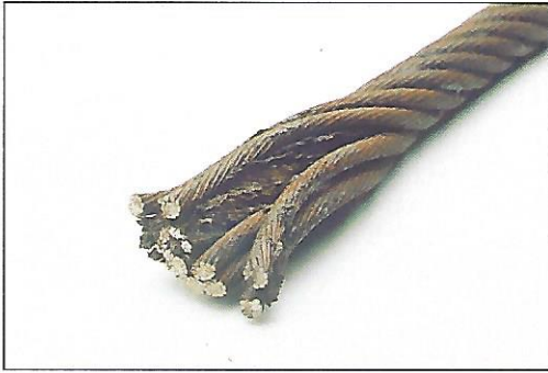
This 7/8" (22 mm) special wire rope, with plastic-coated core, is only 8 months old, rusted through from lack of lubrication. It had to be replaced.
