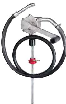
This heavy duty rotary barrel pump has an aluminum die cast body and includes a 2" cast iron bung adaptor and die cast aluminum handle with security locking latch.
